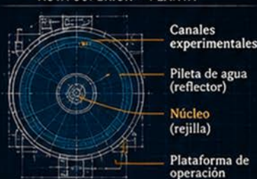
REACTOR EXPERIMENTAL RA-2 VISTA SUPERIOR - PLANTA
